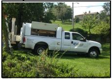
Mounted on a four-wheel drive Ford carrier vehicle, this probe is a versatile and durable machine capable of accessing challenging terrain. The 5410 is equipped with a DT21 Dual Tube Sampling system that utilizes 2.125-inch OD probe rods as an outer casing and 1-inch rods for the inside rod string. A cutting shoe is installed on the leading end of the rod string and allows soil samples to be collected in disposable clear plastic liners.
