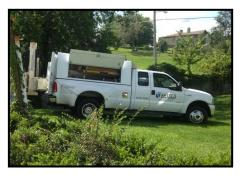
Mounted on a four-wheel drive Ford carrier vehicle, this probe is a versatile and durable machine capable of accessing challenging terrain. The 5410 is equipped with a DT21 Dual Tube Sampling system that utilizes 2.125-inch OD probe rods as an outer casing and 1-inch rods for the inside rod string. A cutting shoe is installed on the leading end of the rod string and allows soil samples to be collected in disposable clear plastic liners.
